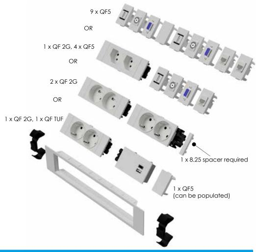
**Configurations:** The QF45 Thick Panel Frame Can be fitted with the following Qikfit module combinations:
